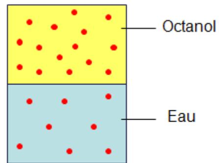
$$K_{ow} = C_{octanol} / C_{eau}$$
