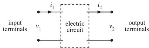
**FIGURE 3** A circuit with input and output terminals.
